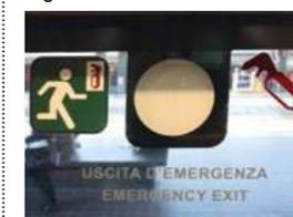
Pick up the hammer for breaking glass (Fig.2) use it to strike the window at the spot marked (Fig.3) and push the window out.
